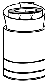
Let the canister slid down the filter slider
