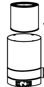
Put in the new hepa filter
